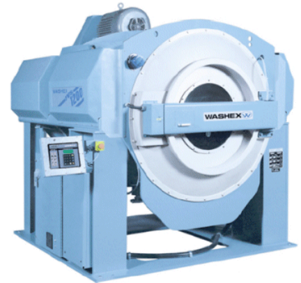
Large open pocket, end-loading washer/extractor
